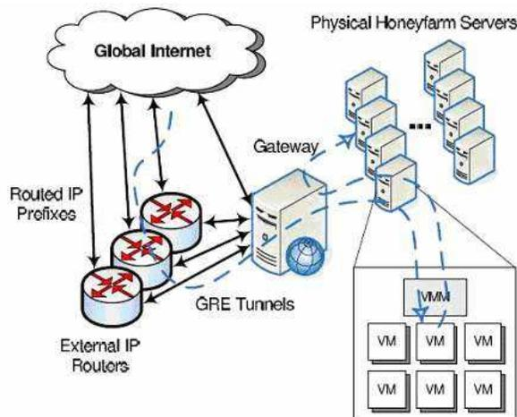
Fig. 1. The architecture of Potemkin [40, Fig. 1].
